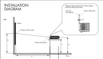
a: Distance between the screen and the centre of the lens b: Distance between the floor and the centre of the lens
